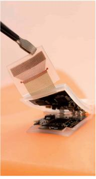
A wearable ultrasonic-system-on-patch for deep tissue monitoring.
