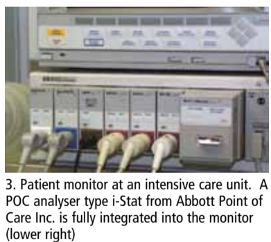
3. Patient monitor at an intensive care unit. A POC analyser type i-Stat from Abbott Point of Care Inc. is fully integrated into the monitor (lower right)
