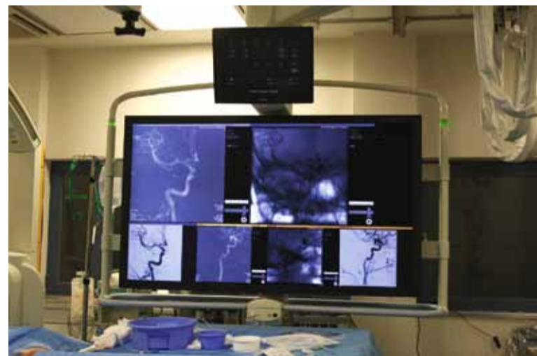
Aneurysm intervention: Configuration for an aneurysm intervention. The working projection is important and thus enlarged, while other images are minimised
