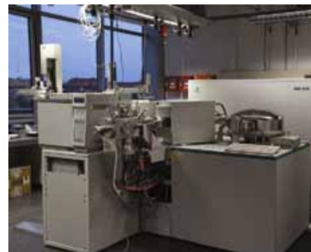
Liquid chromatographic cleansing of probe extract for dioxin and PCB analytic
